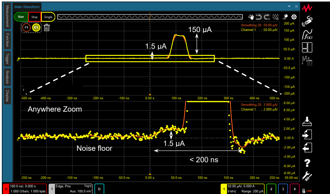
Figure 22. Pulsed measurement example using the pulse generator and CX3300A
